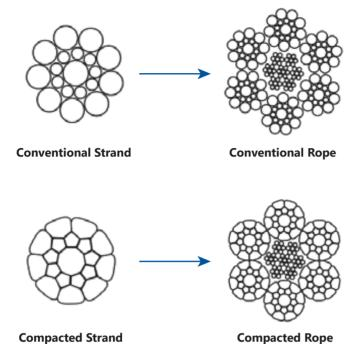
A Powerform® compacted rope is a steel wire rope which has been manufactured using individually compacted strands.
