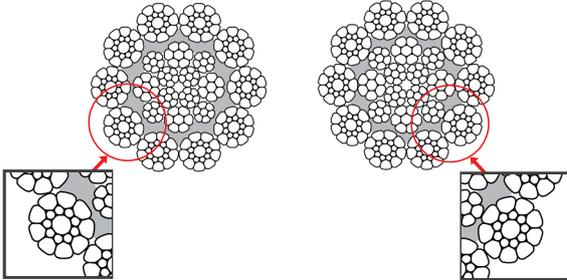
Figure 16 Cushion layer versus plastic impregnated core
