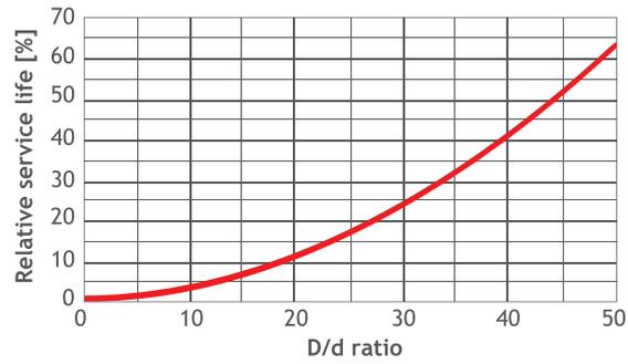
Figure 52 Effect of bending ratio on service life
