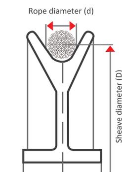
Figure 58 Bending ratio between rope and sheave
