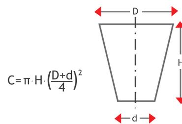
Figure 37 Resin content and cone dimensions
