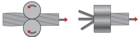
Figure 9 Compacting process through rollers or die
