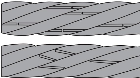
Figure 60 Crown and valley breaks due to fatigue
