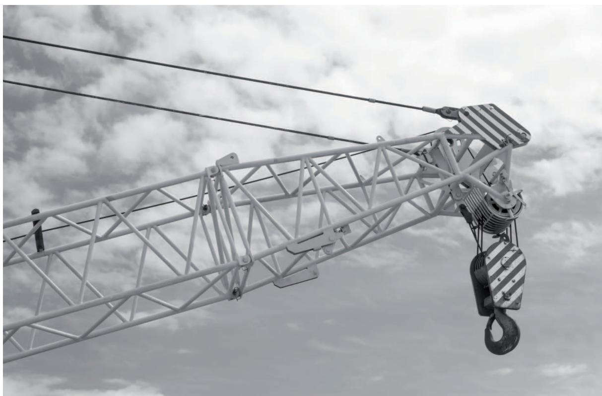
Figure 34 Detail of hoist and boom ropes
