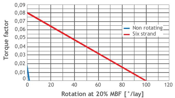
Figure 20 Torque factor for non rotating and six strand ropes
