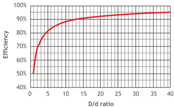
Figure 40 Reduction in rope efficiency in case of bent over stationary components
