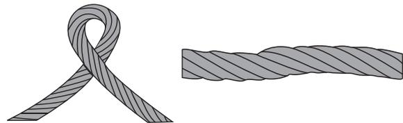
Figure 32 Rope kink and associated deformation
