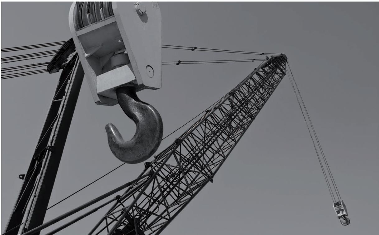
Figure 22 Multiple fall lifting
