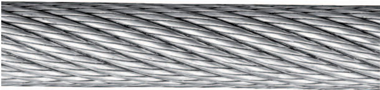
Figure 26 Example of rope with very low outer lubrication
