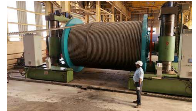
Oceanmax: 180-tonnes single rope produced at Ranchi unit
