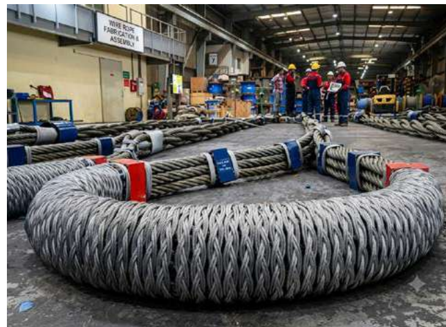
228 mm Engineered Grommets for heavy-duty lifting
