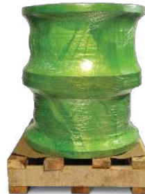
Stretch wrapping the polyethylene-covered reel.
