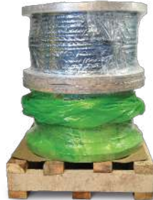
Setting the reel on a wooden pallet and covering it with a polyethylene bag.
